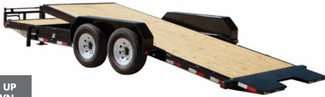
20 ft 6" Channel Tilt (T6) Pictured (4' Stationary Deck + 16' Tilt)
