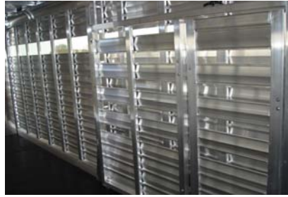
1" x 3" tubular uprights/extruded sides
